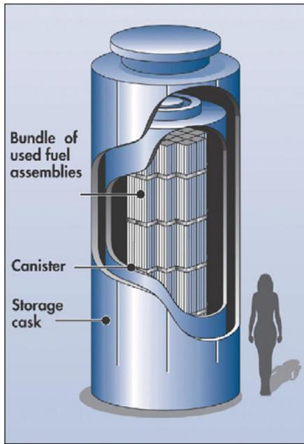
Dry Cask Storage Cutaway
