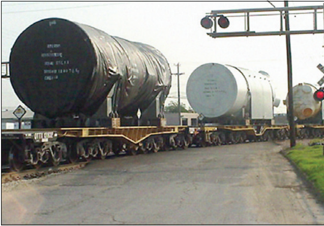
Large Component Transportation Rail shipment utilizing special shielding and packaging requirements
