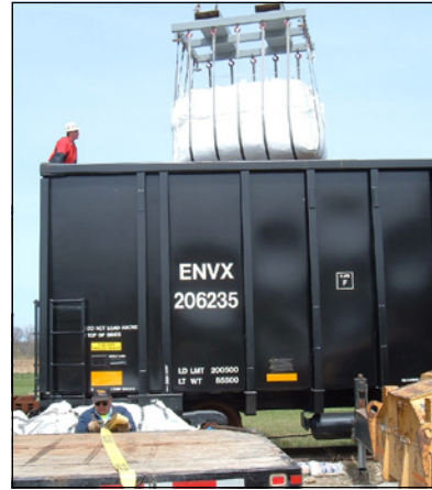
Waste Loading Loading SuperSacs in EnergySolutions' supergondola railcars
